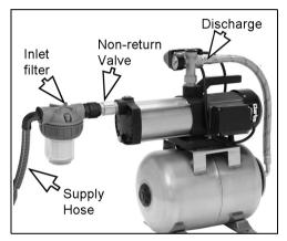
Where the pump is to be a permanent fixture, the fittings to the pump MUST be flexible, i.e. a short piece of hose should be inserted between any rigid metal pipework and the pump.
