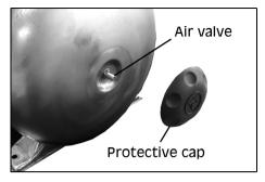
Check the air pressure gauge until satisfied and replace the protective cap when completed. This procedure MUST be carried out before connecting to the water supply.
